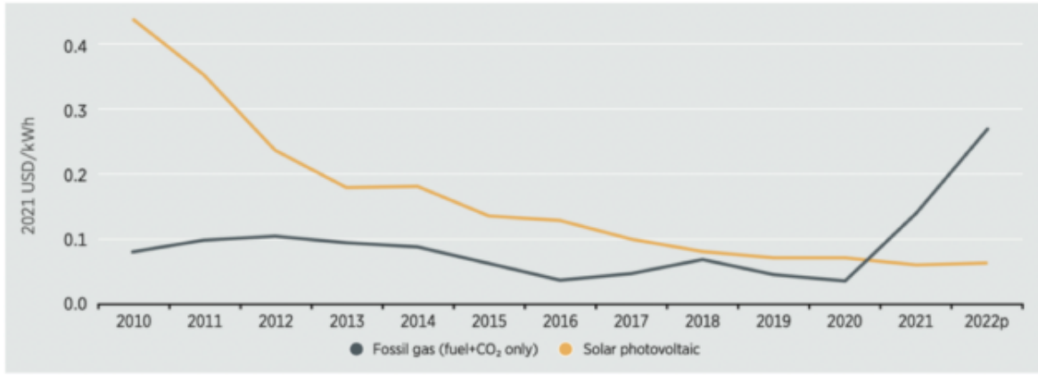
Figure ES.3 The weighted average LCOE of utility scale solar PV compared to fuel and CO 2 cost only for fossil gas in Europe, 2010-2022
