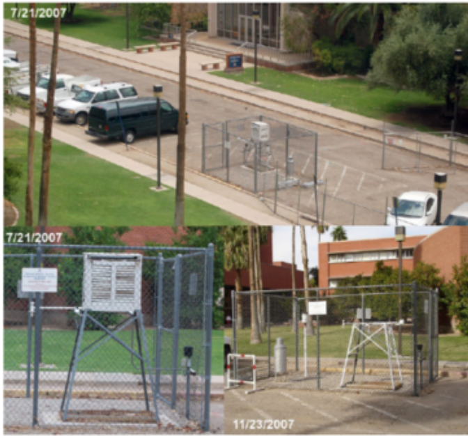
Figure 8: Top: placement of CRS in parking lot at University of Arizona Atmospheric Sciences Department on July 21, 2007. Lower left: detail at ground level of CRS placement on July 21, 2007. Lower right: detail at ground level of CRS after removal on November 23, 2007. Source: Warren Meyer, Bob Thompson.
