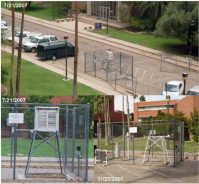
Figure 8: Top: placement of CRS in parking lot at University of Arizona Atmospheric Sciences Department on July 21, 2007. Lower left: detail at ground level of CRS placement on July 21, 2007. Lower right: detail at ground level of CRS after removal on November 23, 2007. Source: Warren Meyer, Bob Thompson.
